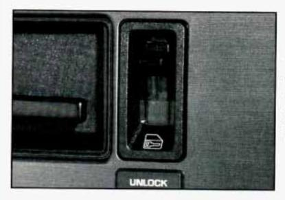
From the inside: To lock front doors and sliding side door, slide the lock levers down.
